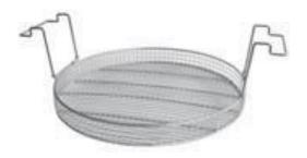
Insert basket K 40 stainless steel Dia. 480 mm, 50 mm high mesh width 12.5 × 12.5 mm max. load 10 kg Code No. 123
