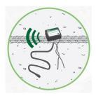
SmartRock2 is a rugged, waterproof, wireless sensor that allows to control the real-time temperature and maturity of concrete. The sensor is installed on the rebar placed in the concrete formwork before pouring. Using the SmartRock2's smartphone/tablet app for monitoring the maturity of the concrete and sharing the data is easy and quick.
