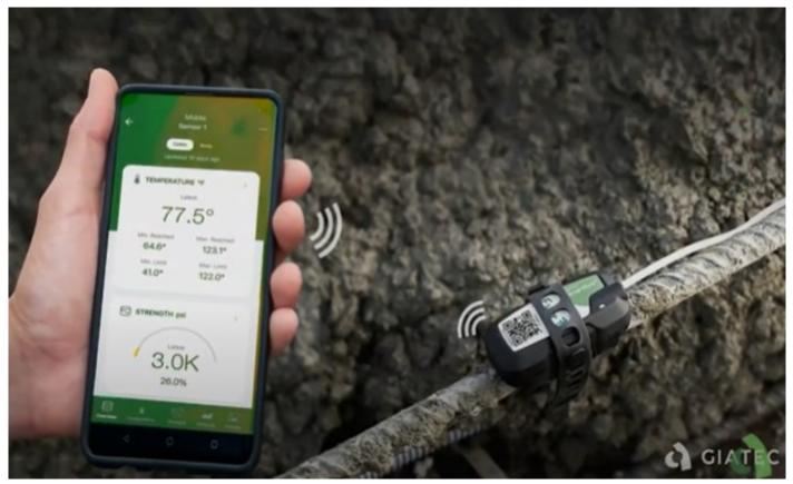
SmartRock is the world's leading wireless sensor for monitoring the curing and hardening of concrete. The sensor is fully-embedded and secured on the rebar, making it completely maintenance and hassle-free.
