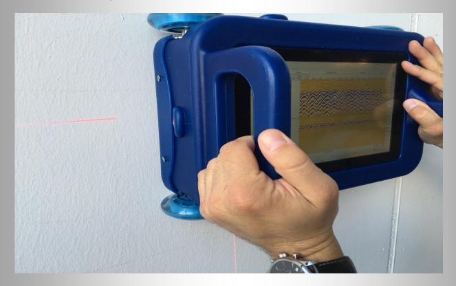
Quantum Mini Radar is a rugged, wireless and hand-held scanner for inspection of walls, bridges and other concrete slabs. The technology used in Mini Quantum integrates at the same time:
