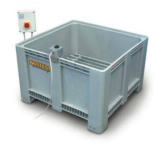
Made from extremely robust and stable polyethylene, complete with base rack from polyethylene. Supplied with analogic thermostat heating system and stop cock. Tank can conserve more than 100 concrete specimens with dimensions 15x15x15cm<sup>3</sup> under water at a temperature of 20 °C +/- 2°C.
