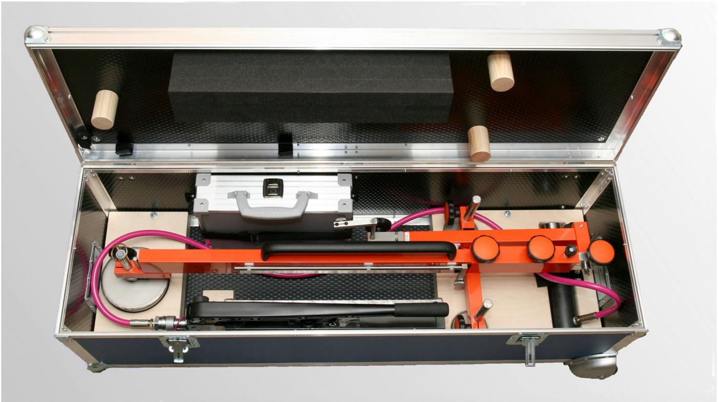
Thanks to this solution reading of the results is quicker and simplified. Additionally, the thermal printer built into the device provides an immediate printout of the measurement data. The results are shown in a diagram that may be helpful for interpreting test results.
